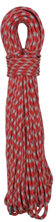
CMC G11 Lifeline is the first NFPA, G-rated 11 mm rope made from traditional fibers. It is a low-stretch kernmantle rope constructed with a polyester sheath and nylon core. G11 Lifeline offers maximum strength in a lightweight and easy to handle rope. Providing enhanced safety and performance, as well as superior knotability, it is ideal for rope rescue and rope access operations.
