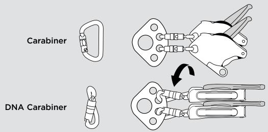
The CMC DNA ANSI Carabiner enables 90° rotation of any connected device for offset load management including descenders, progress capture devices, rope clamps, and fall arresters. When used in the Double CLUTCH TTRS, the DNA optimizes CLUTCH handle alignment to allow a single operator to manage both CLUTCH handles for simultaneous twin tension control. The Double CLUTCH TTRS hauling/lowering system meets best practices, minimizes failure risks, and has the potential to reduce personnel needs.
